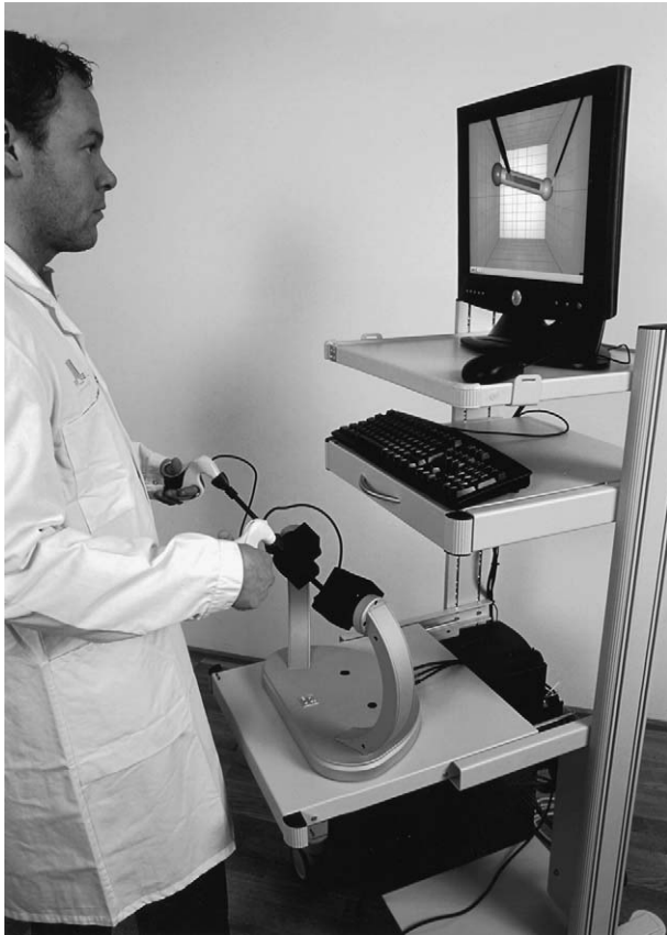
Fig. 2. The Procedicus MIST trainer simulates laparoscopic surgical techniques through visual and haptic interfaces. (Photo courtesy of Mentice, Gothenburg, Sweden.)
