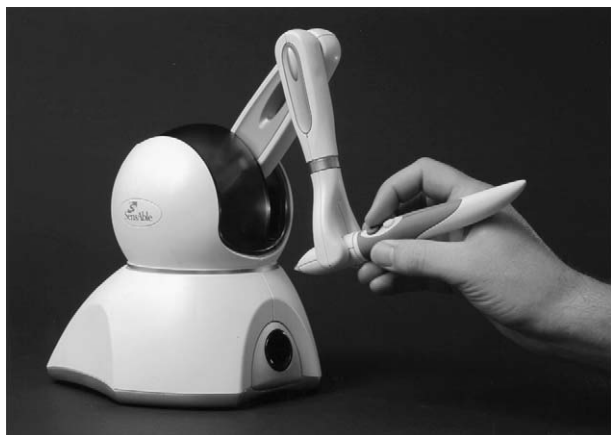
Fig. 10. The PHANTOM haptic feedback device is an example of a haptic display device. (Photo courtesy of SensAble Technologies, Inc., Cambridge MA, USA. PHANTOM, PHANTOM Desktop, SensAble, and SensAble Technologies, Inc. are trademarks or registered trademarks of SensAble Technologies, Inc.)
