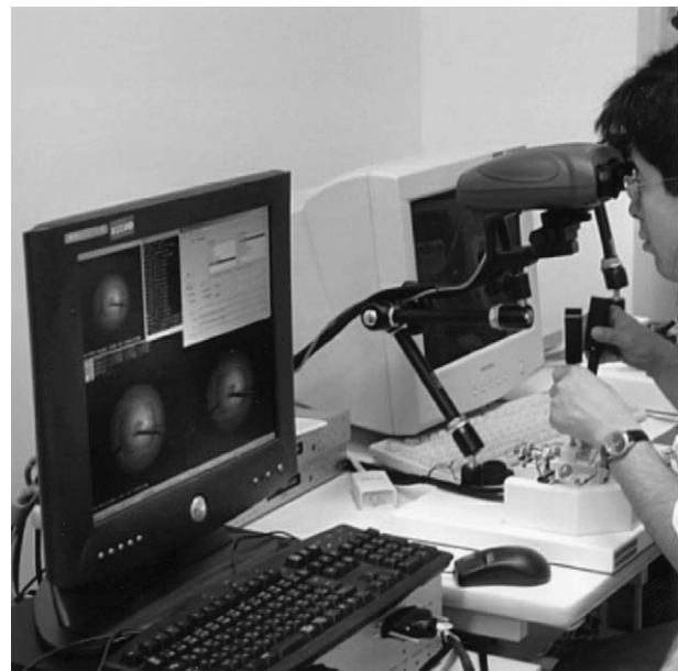
Fig. 5. Vitreous surgery simulator hardware setup developed in 2000 by the Department of Ophthalmology at Asahikawa Medical College, Japan. (Photo courtesy of Taiichi Hikichi, MD, Asahikawa Medical College, Japan.)
